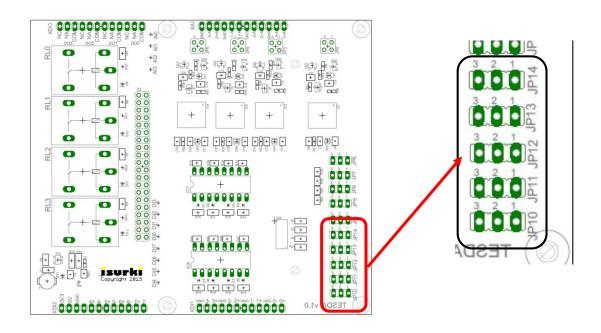
Jumpers 10, 11 and 12 allow to select if the first three of the four configurable digital points will work as input or output. Shortcircuiting the pins 1 and 2 of the jumper configure the point as input. On the other hand, connecting the pins 2 and 3 will configure the point as an output. To summarize:
