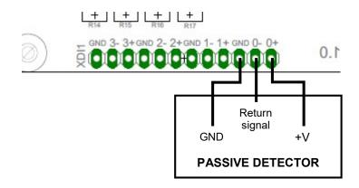
In the above mentioned example, the 18 Vdc excitation to the detector is given through the 0+ and GND pins of the board. The output signal of the detector inputs the board through the 0- pin. For the rest of digital inputs, the diagram is equivalent.
