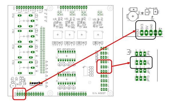
In case of using both auxiliary sources at the same time, the ground (GND) terminal should be shared.
