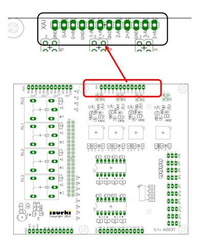
The connection procedure of a 4-20 mA current loop sensor is different depending on if it requires external excitation (passive sensor) or not (active). For the first case, the TESDA board provides a high quality industrial 18 Vdc auxiliary supply. The next drawings illustrate this concern, based on the first analogue channel marked as AIO.
