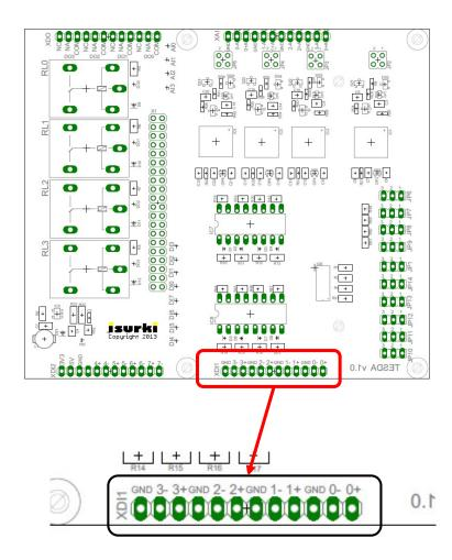
These digital inputs allow the connection of industrial field devices such as voltaje free contacts, passive and active detectors (photocells, inductive detectors, ...), ...
