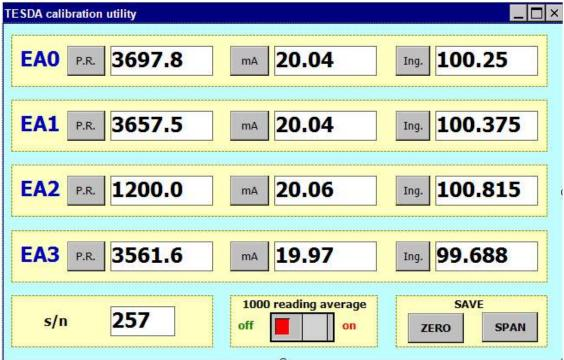
Using the ZERO and SPAN buttons located at the bottom right of the window the user can save the calibration results into a text format file.
