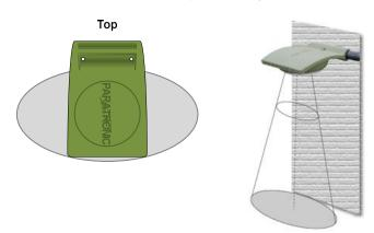
To use the self-positioning feature, the shipping seal must be removed from the Cruzoé Radar (rubber cord [black] inserted between the shell [green] and the aerial [white]).
